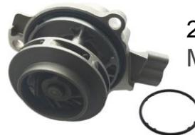
2) Fit the new SKF Mechanical VKPC 81178
