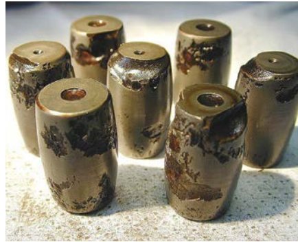
Rollers from a counterfeit spherical roller bearing
